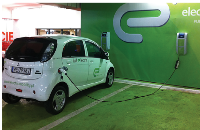
Electric automobile recharging
